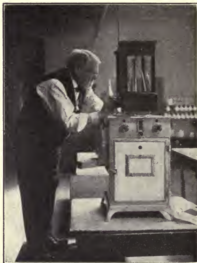
Weighing Cotton Yarn Inside an Oven for Customs Determinations
